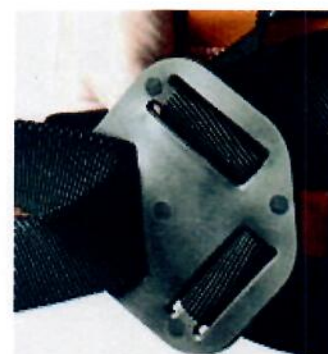
the back D-Ring pad is not damaged or cracked
